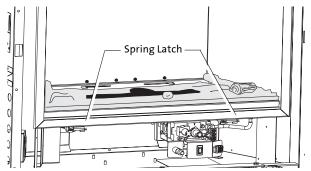
Pull each Spring Latch to disengage them from the Glass Frame.
